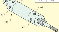
This option is used in applications where ports need to be rotated to accommodate a specific space requirement or port orientation for the fittings and tube attachments. The diagram explains the options and orientation of the ports. See the specific cylinder to find availability of these options.
