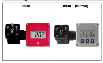
The 8930 and 8930T are microprocessor controlled display devices for 4 - 20 mA standard signals that can be universally applied. They do not require an auxiliary voltage source but can be supplied directly from the measuring current.
